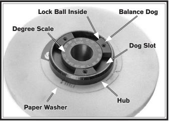
Figure 40. Grinding wheel hub.
